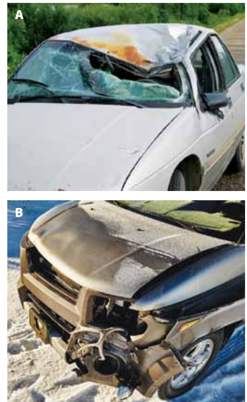
FIGURE 3. Typical principal points of contact between animals and vehicles following moose–vehicle collisions (A; 6 July 2005) and deer–vehicle collisions (B; 2 January 2015).
