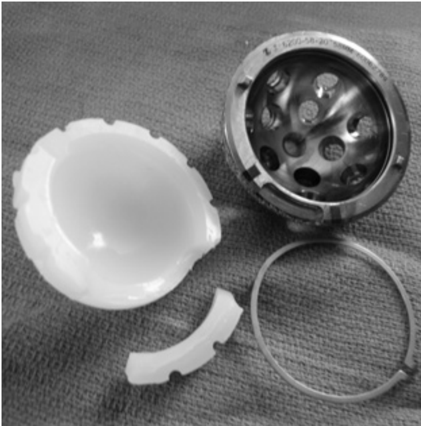
Figure 8. Fractured rim of a cross-linked polyethylene liner. The acetabular component was placed in a vertical orientation, leading to a fatigue fracture at the superior aspect of the polyethylene liner.
