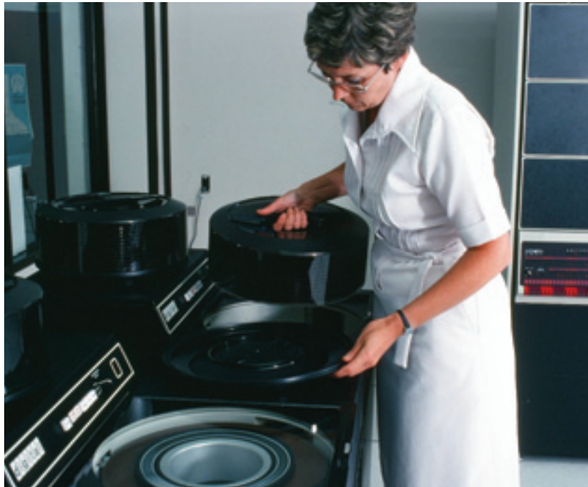
An early photo from the 1970s of a staff member replacing one of the storage "drums" that were used for backups.
