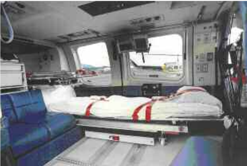
Figure 2. Interior of Bell 222 helicopter. Notice the pilot's seat directly in front of the patient's stretcher and the proximity to the paramedic attendants. The patient is immediately adjacent to the helicopter door, which cannot be locked for safety reasons.
